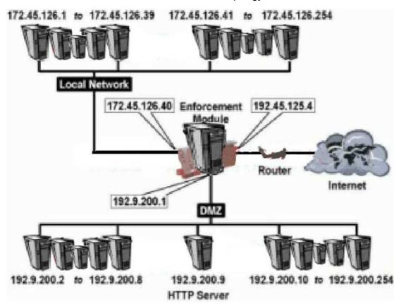
You want hide all localnet and DMZ hosts behind the Enforcemenet Module, except for the HTTP Server (192.9.200.9). The HTTP Server will be providing public services, and must be accessible from the Internet.
