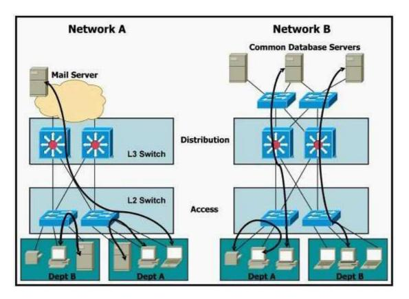
A. Network A is designed to accommodate file transfers from other department servers on a frequent basis.
