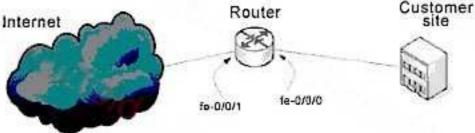
In the exhibit, after applying the firewall filter to the router, the customer notices that some unwanted ICMP traffic is still passing through the router.
