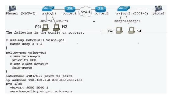
A. It is NOT possible to configure multiple DSCP matches in one statement under 'classmap'. So, the packets that are marked as DSCP=5 by IP phones are not going through priority queue. Instead, it is going through 'default queue '. So, IP phone packets are getting delayed. Thus, it caused the voice quality problem.
