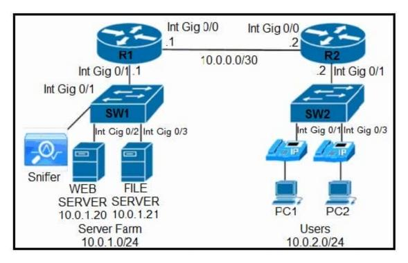
A network engineer is troubleshooting an issue with the file server based on reports of slow file transmissions. Which two commands or command sets are required to switch SW1 to analyze the traffic from the file server with a packet analyzer? (Choose two.)
