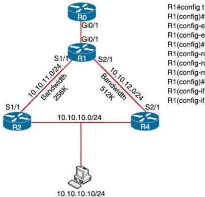
R1(config)#ip access-list extended UDP-ACL R1(config-ext-nacl)#permit udp any any R1(config-ext-nacl)#exit R1(config)#route-map VIA-R2 permit 10 R1(config-route-map)#match ip address UDP-ACL
