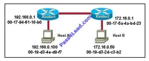
Host A is sending a packet to Host B for the first time. What destination MAC address will Host A use in the ARP request?
