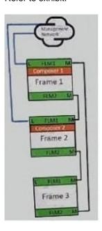
You are installing three Synergy frames for a customer PoC in the configuration shown. The composer ids unable to discover the frames What is the mostly likely cause of the problem?
