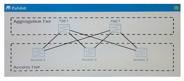
Referring to the exhibit, you are designing a Layer 2 data center and you want to make sure that all the links between the access tier and the aggregation tier are used.
