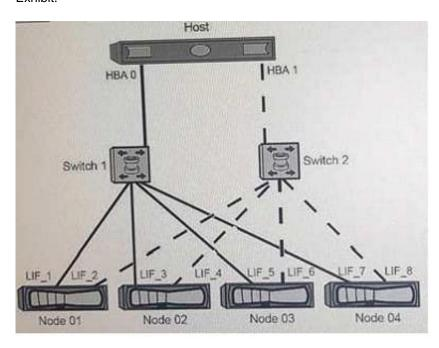
A customer is testing a dual-fabric FC SAN configuration as shown in the exhibit. The zones are implemented on the switches shown below.
